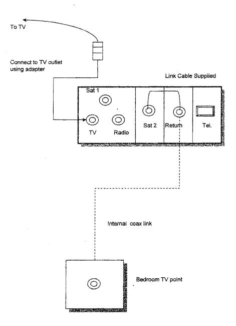
The cable supplied can be used as either a Satellite link or the "return" feed by using the adapter/s supplied
